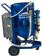
The pressure pot is a key component of the Farrow System®. Specifically sized for the output of the machine, each pot complies with ASME vessel code regulations Section VIII, Division One. Each pot is powder coated inside and out to assure maximum reliability and longevity in the field.
