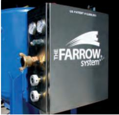
The 100% stainless steel control cabinet is super durable and sealed against the elements. It houses the dosing regulators, controls, valves, and gauges that monitor the system performance. Intuitive controls are easy to use, reducing training time required to get consistent results.
