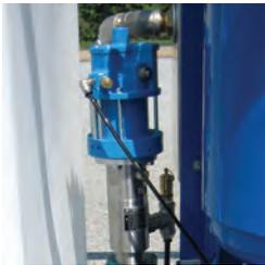
Compressed air is used to pump water for the process from an on-site water source.
